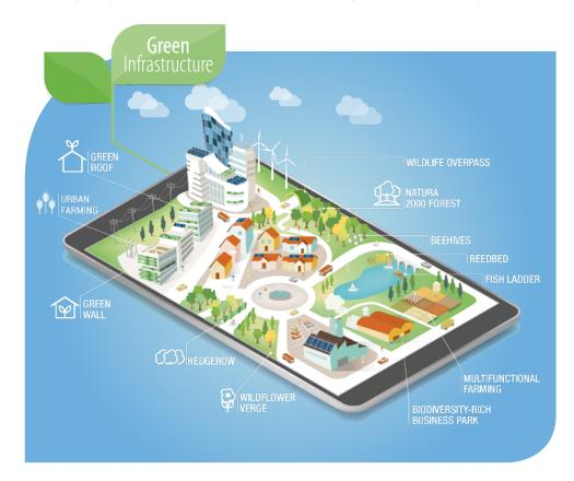
walls or green embankments along infrastructure function as noise barriers, reduce air pollution through particulate filtering, mitigate water run-off as well as reduce storm-water flows as part of a sustainable drainage systems. Elements of Green Infrastructure that can be integrated into road construction include vegetated drainage in combination with porous materials, permeable pavers, into streets or parking lots. These measures increase on-site neighbourhood storm water capacity.
